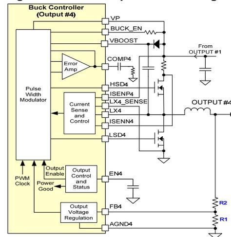
**Figure 7 - Power Output #4 Block Diagram - BOOST**
