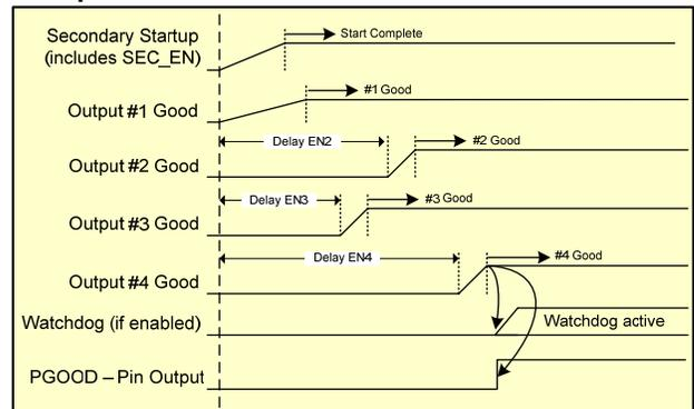
Figure 12 - Hardware Mode PGOOD Generation
