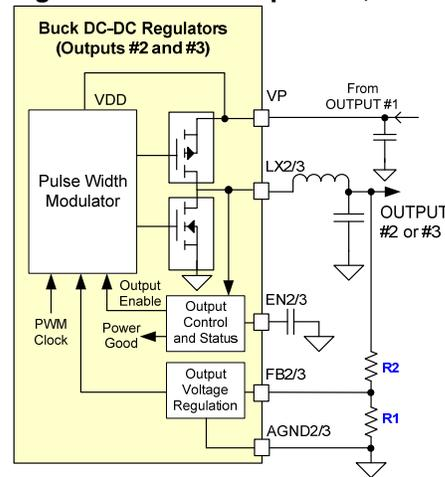
Secondary-side Outputs #2 and #3 (see Figure 5) are identical synchronous current mode PWM DC-DC Buck Regulators with:
