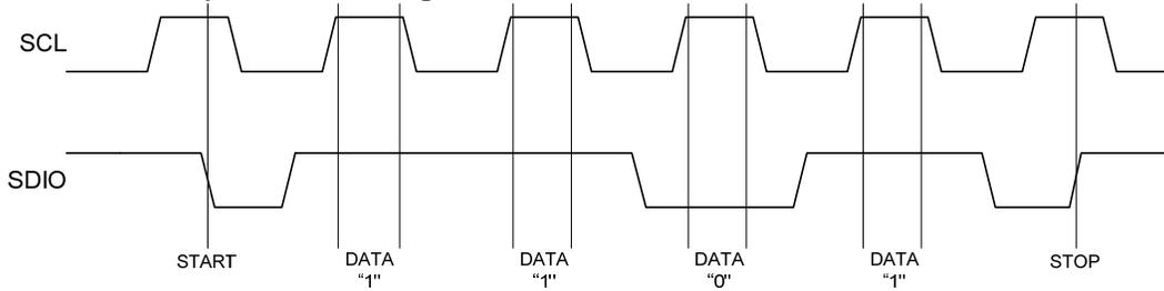
Figure 20 - I<sup>2</sup>C Acknowledge Timing
