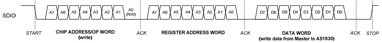
**Figure 23 - I<sup>2</sup>C Interface Read Cycle Timing (with Repeated Start)**
