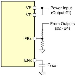
Figure 10 – HW Mode Output(s) Hardware Disabled
