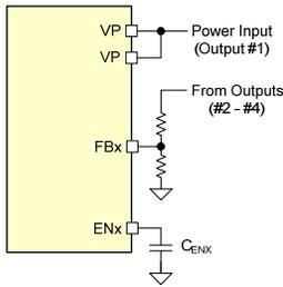
**Figure 15 – SW Mode Output(s) Hardware Disabled**
