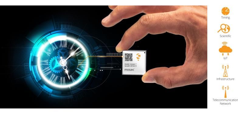
Septentrio mosaic-T<sup>™</sup> is a **multi-band**, **multi-constellation GNSS timing receiver** designed specifically for providing the highest security and availability for critical infrastructure and other applications where resilient timing is essential.
