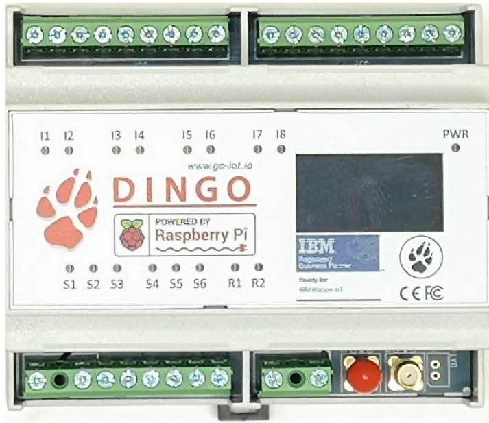
DINGO 2-Station Gateway with terminal covers removed showing Antenna SMA connectors (one with red protective cover)
