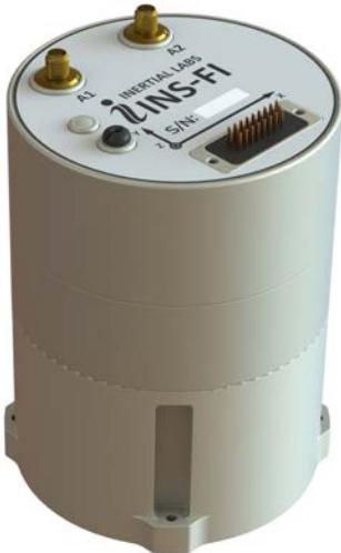
Due to its high-performing FOG IMU, the **INS-FI** can measure GNSS-free Heading (True North) with less than 0.5 deg error, Horizontal & Vertical Positions with approximately 0.1% error of Distance Traveled for land applications, and 5 nautical miles per hour drift for aerospace (Unmanned Aerial Vehicles) applications without GNSS signal.
