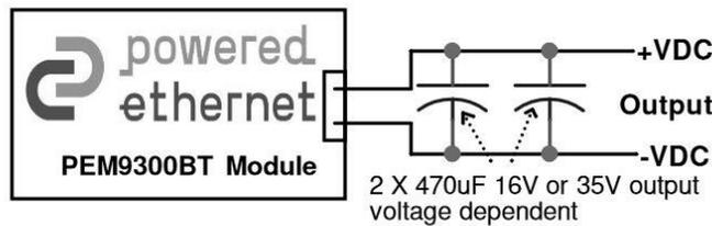
Figure 2- Output connection
