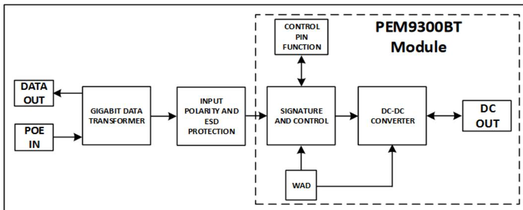
Figure 3- Block Diagram
