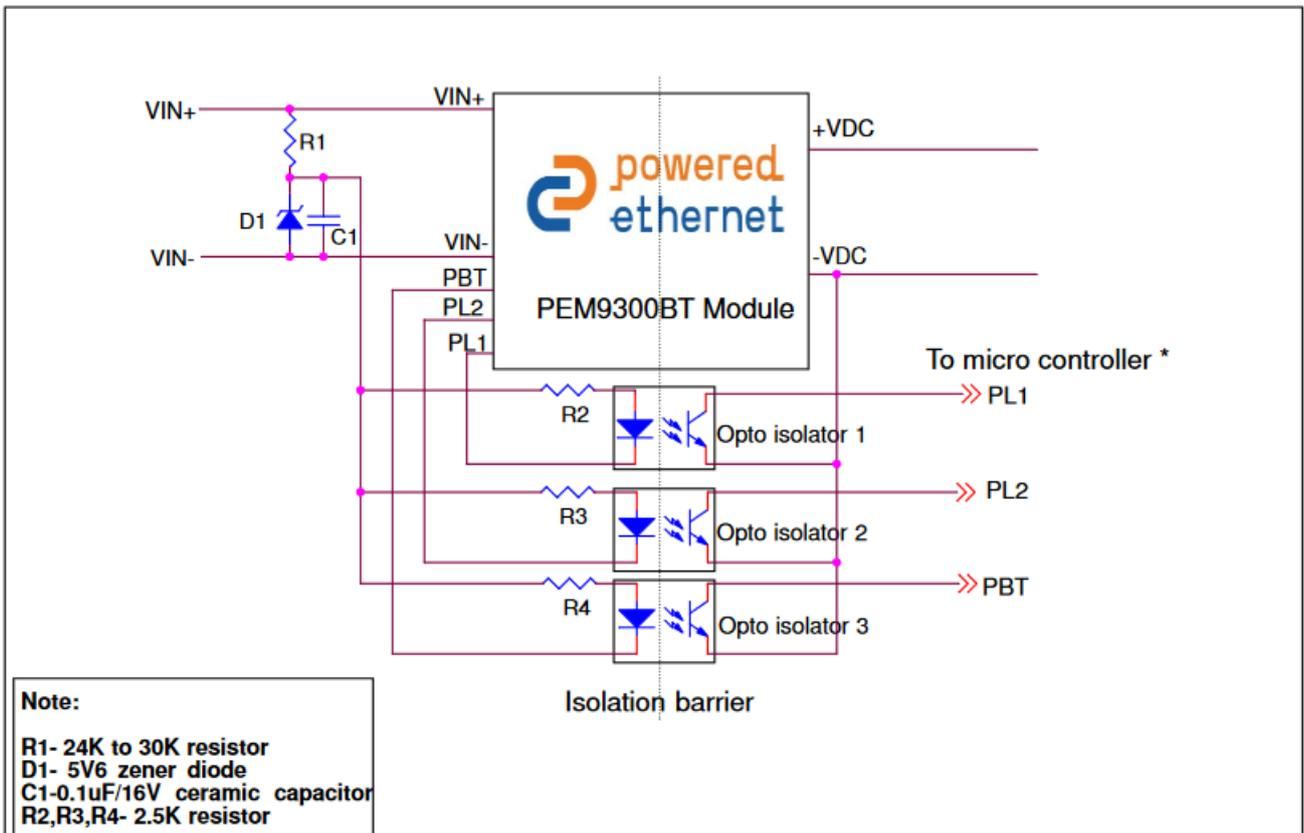
Figure 4- Power level indication connections to host-board
